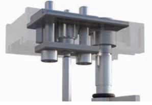
STEP 4 Adjust pivot door with Tomma T Bar by rotating the centre adjustment screw as shown, either clockwise or anti clockwise
